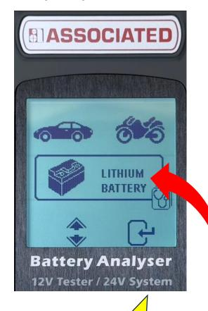
Also allows for 12 & 24V Alternator, Starter, and Ground **System Testing**
