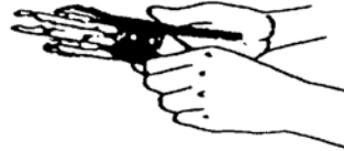
Extended position Note: Pressure, when handle is squeezed, holds adapter firm. Will not slip back.
